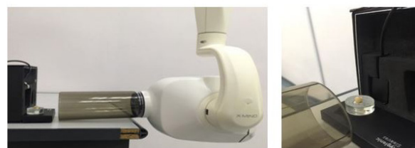
Figure 3: Contrast medium (Iopamidol®) was left for 5 minutes on the occlusal surface of the tooth before IOPA was taken. Paralleling technique for imaging the sample was used in this study.
