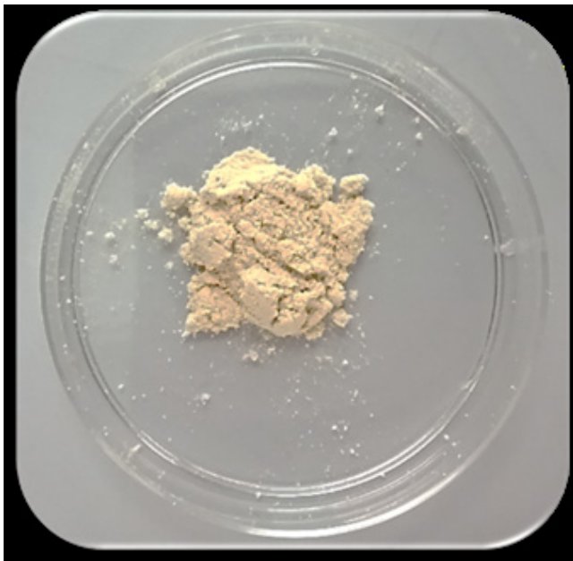
Figure 3: M.oleifera Leaf Extract of Deionised water. The aqueous extract of the M.oleifera leaf after freeze drying appears as an off-white coloured powder.
