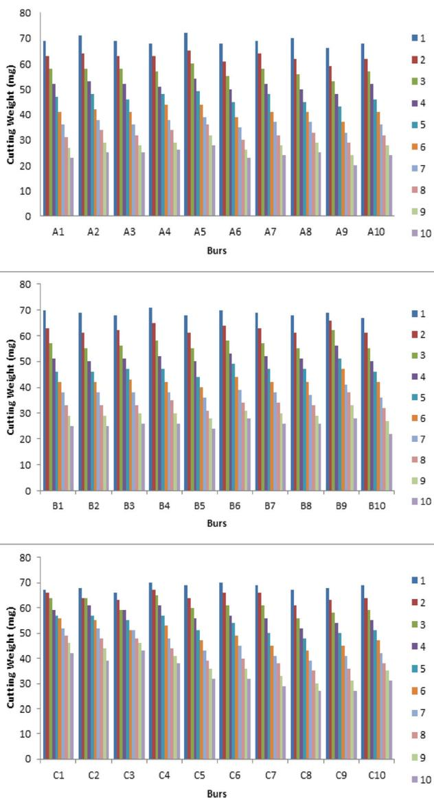
Figure 3: Sample’s weight-loss of the first cut (1) to the tenth cut (10) for each bur in Group A, Group B, and Group C
