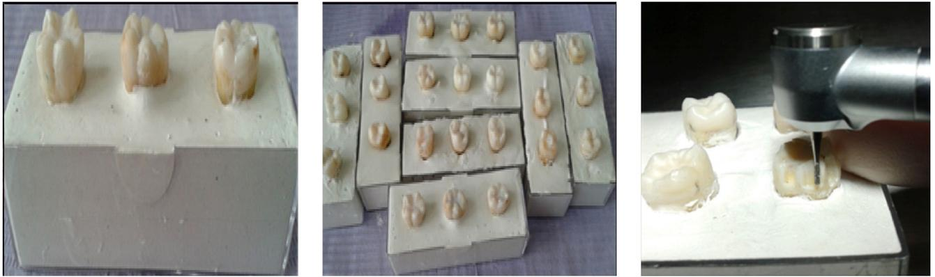
**Figure 1:** Teeth samples moulded into a block and the cutting procedure
