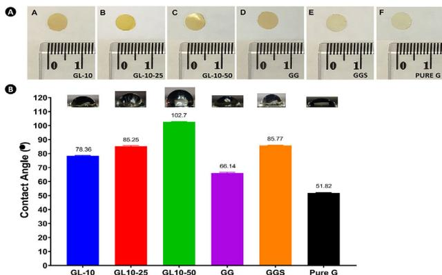
Fig 4: Biomaterials Characterization of different films. (A) Gelatin-Spidroin Films Visual Aspects and (B) Contact Angle Analysis.
