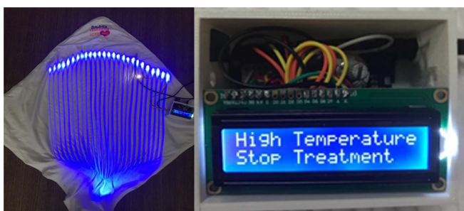
Figure 3a and 3b : Prototype of the operational Smart Biliwrap system during testing.
