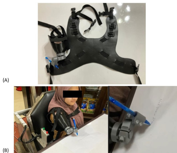
Figure 3 : Fabrication and testing process (A) The socket was supported with a harness to allow better fit and adherent to the patient’s limb and prevent the socket from loose off the limb. (B) The patient fit well with the devices and manage to write on the first trial
