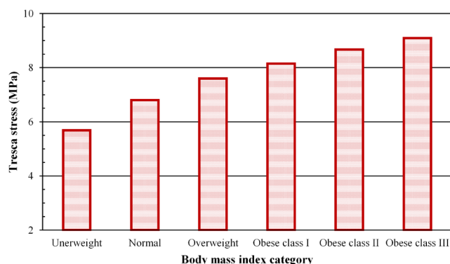
Figure 4 : Tresca stress magnitude of CoCrMo-on-UHMWPE bearing at peak loading under normal walking condition from various categories of body mass index.
