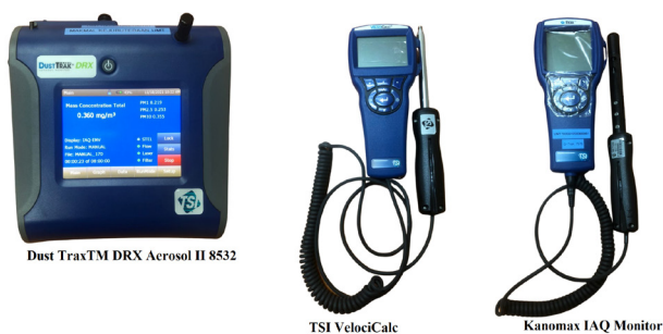
Figure 2: Instruments used for data collection. Instruments used to include Dust TraxTM DRX Aerosol Monitor 8534, Kanomax IAQ Model 22b11, and TSI Climomaster Model 9545.
