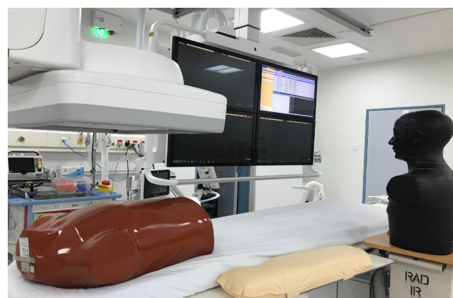
Fig. 1: Phantom setting. The Anthropomorphic Thorax Phantom representing the patient was laid on the angiography table, and the Alderson-Rando (A.R.) Phantom, representing the cardiologist, was placed on the trolley table with a height set to meet the average adult. The A.R. phantom stood 35cm to the right of the Anthropomorphic thorax phantom.
