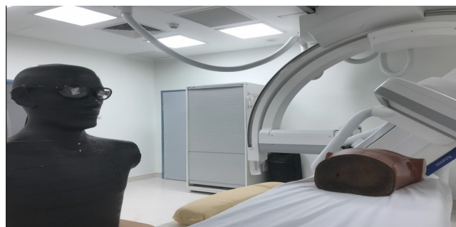
Fig. 3: The setting of the lead eyeglass shielding on the A-R Rhando phantom. The lead eyeglasses, weighing 76g with a lead equivalent of 0.75 mm Pb, are placed to provide shielding to the lens of the eyes.
