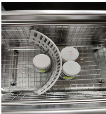
Fig 1: Sonication of fMWCNTs nanoparticles in various solvents
