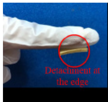
Fig. 2: PVA/Gel/NaCl0 with 3% TA detached at the edge
